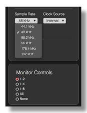
Your Scarlett interface is able to operate at any of six sample rates: 44.1 kHz, 48 kHz, 88.2 kHz, 96 kHz, 176.4 kHz and 192 kHz. The default sample rate is 48 kHz. Select an alternative sample rate if needed. Note that the optical input is disabled when sample rates of 176.4/192 kHz are in use.
