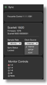
Interconnected digital audio equipment must always use the same reference clock source. Your Scarlett interface is able to synchronise from three sources:
