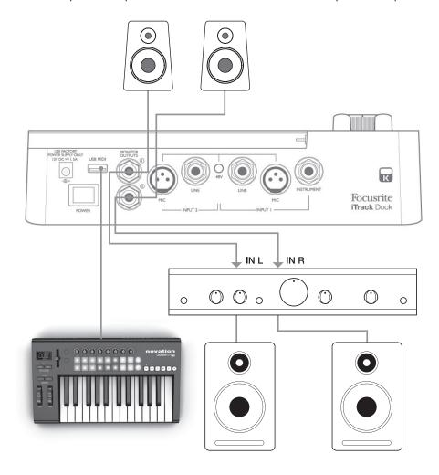
The line output connectors are 3-pole (TRS)  $\frac{1}{4}$ " (6.35 mm) jack sockets, and are electronically balanced. Typical consumer (hi-fi) amplifiers and small powered monitors will have unbalanced inputs, either on phono (RCA) sockets, or via a 3.5 mm 3-pole jack plug intended for direct connection to a computer. In either case, use a suitable connecting cable with jack plugs at one end.
