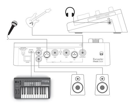
This setup illustrates the most typical configuration for using a recording app. Here, you might record guitar through Input 1 and vocals through Input 2 into your preferred app, while monitoring the playback – anything you've already recorded - via headphones or loudspeakers.
