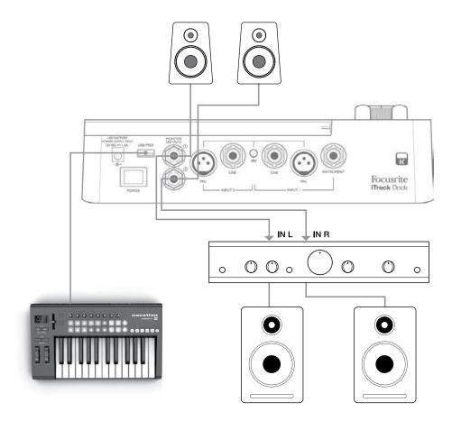
The **MONITOR OUTPUT** connectors are 3-pole (TRS)  $\frac{1}{4}$ " (6.35 mm) jack sockets, and are electronically balanced. Typical consumer (hi-fi) amplifiers and small powered monitors will have unbalanced inputs, either on phono (RCA) sockets, or via a 3.5 mm 3-pole jack plug intended for direct connection to a computer. In either case, use a suitable connecting cable with jack plugs at one end.
