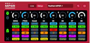
The illustration above shows the RedNet MP8R RedNet Control image. The signal level, gain and input function settings are indicated for each channel. Use the Live and Setup buttons at the top of the graphic to change view.
