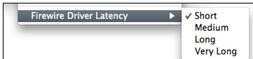
If you are experiencing clicks and pops or audio dropouts, this may be due to certain hardware in your computer that is affecting the performance of audio devices connected via FireWire. Rather than removing and replacing hardware (e.g. your graphics card or wireless internet card) trying a longer Firewire Driver Latency setting may solve the problem.
