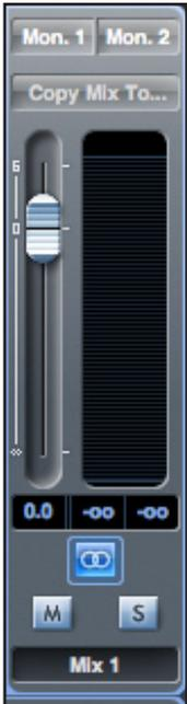
The output channel can be either mono or stereo depending on the status of the stereo button. When the channel is set to stereo, you will see that the tab for that mix doubles in size. This is due to the fact that the stereo version takes up 2 channels of the available total output channel count.
