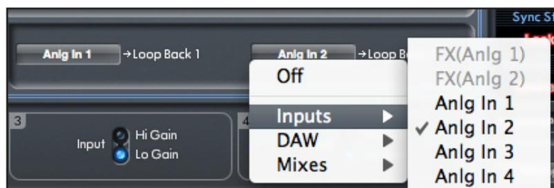
When 'Anlg In 1' and 'Anlg In 2' are routed to Loopback, these will be available to record in your DAW via the Loopback input channels.
