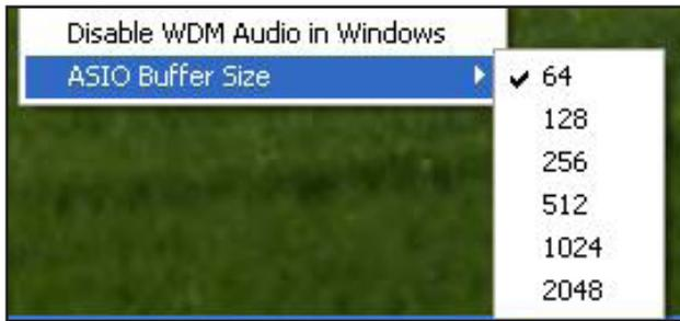
A small buffer size will result in lower latency at the expense of increased CPU usage. A high buffer size will result in a higher latency but with lower CPU usage. If you are using lots of virtual instruments and effects processing in your DAW project, and the CPU usage is high, then increase the buffer size to permit lower CPU usage.
