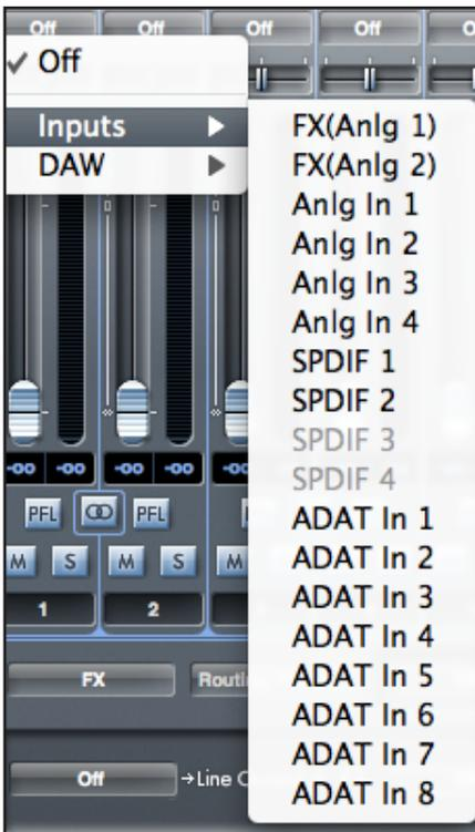
Clicking on the "Off" region brings up a list of all available inputs that can be fed to the channel. All analogue (labelled 'Anlg') and digital inputs, and DAW outputs are available.
