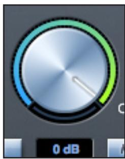
Set the output level of all assigned outputs using this knob. The output level can be adjusted using the mouse and will affect all assigned outputs (as indicated with a blue button). The dB display below shows the current level to which the monitor knob is set.
