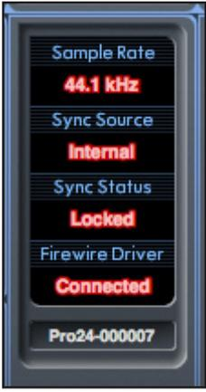
The Device Status section shows information about the sample rate, synchronisation and driver status of the Saffire PRO 24 DSP. The desired sample rate can be set as well as external synchronisation options for using the Saffire PRO 24 DSP with external digital devices.
