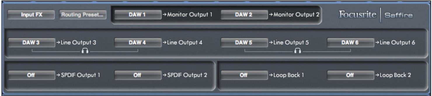
The routing section displays every physical output on the Saffire PRO 24 DSP and the audio stream to be sent to that output is available for selection in a drop down menu to the left of that output.
