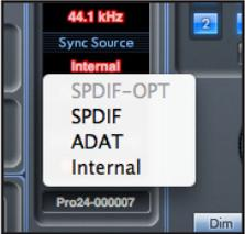
Displays the currently selected sync source (red display) – To change the sync source, click on the red sync source value and select SPDIF -OPT, SPDIF, ADAT, or Internal.
