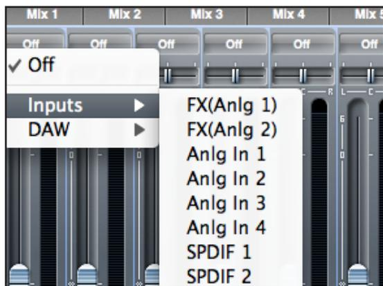
When selecting an Input source in the Mixer or Routing section, the dry signal is represented by 'Anlg In 1' and 'Anlg In 2', and the wet signal as 'FX(Anlg 1)' and 'FX(Anlg 2)'.
