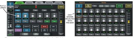
Figure 4.7c: Aux1-2 are linked, Ch01 sent to Aux1-2 and assigned to Main mix
