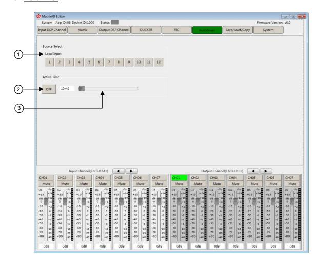
The **Automixer** automatically reduces the level of a microphone when it is not being used. Consequently it lowers the rumble, reverberation and other extraneous noise that occur when several microphones operate simultaneously.
