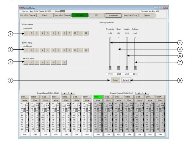
The principle of the **Ducker** is to attenuate one or several channels when priority signals are activated. The main applications are automatic speech for conference or priority messages.
