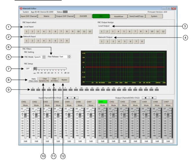
**FBC** or **Feedback Canceller** is a function which eliminates feedback automatically. Feedback occurs unexpectedly in a system where there are microphones and speakers nearby one of the other. This loop effect is an electro-acoustic resonance which generates an unpleasant frequency noise.
