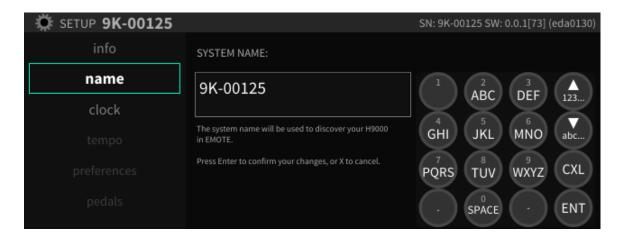
The *Name* screen allows you to create a custom name for your H9000. With custom names assigned, you can easily select the desired unit when using multiple units at the same time and controlling them with emote.
