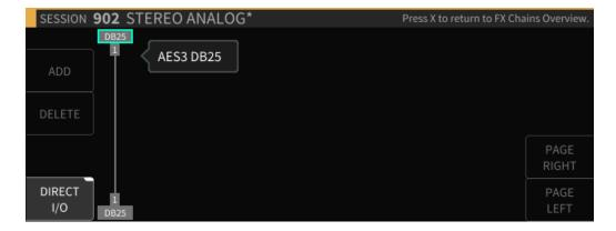
In the Direct I/O screen, use the cursor keys to highlight the input/output you wish to assign, then use the wheel to select the physical input /output you wish to use in your direct I/O pathway.
