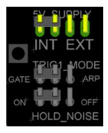
Above: no external 5v supply is required AY3 will provide 5v from the 12v (80mA) rail
