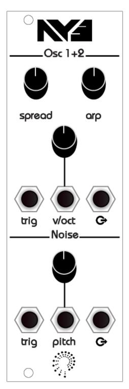
Osc 1 & 2 are detuneable square waves with volt/oct tracking, that can be switched or arpeggiated.
