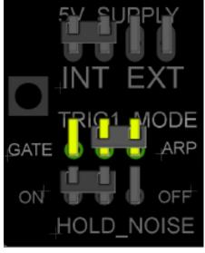
Arp Mode: clock the Arp/switch
