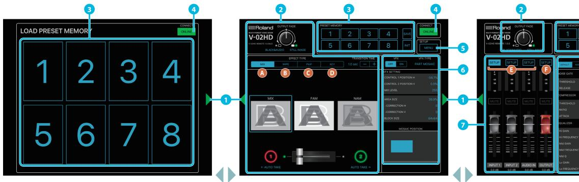
Tap the display-change button (1) to switch left or right through the screens.
