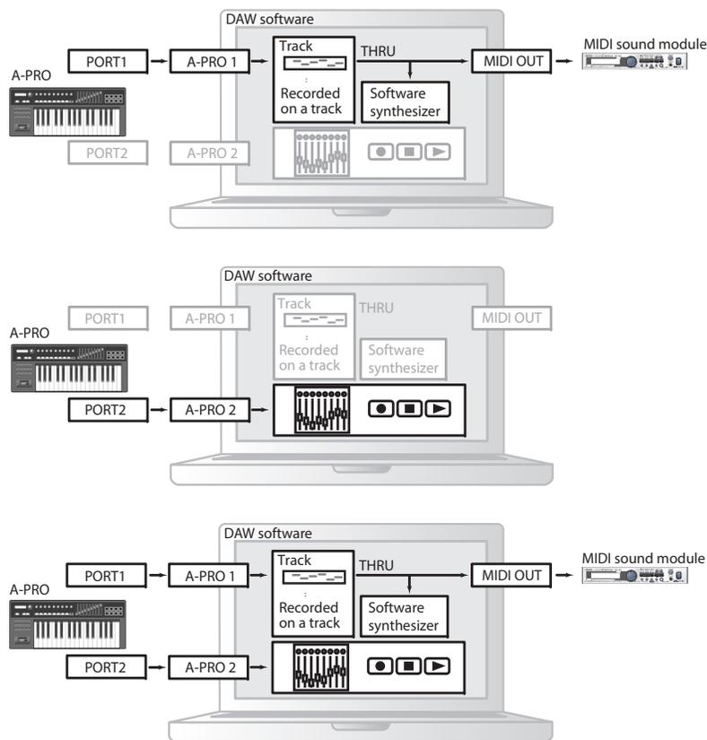
If you're using DAW software, and you're simply controlling the sound module for the part that's producing the sound, the A-PRO's controllers can use the same MIDI output port as the keyboard. When the A-PRO is in the default state, the A-PRO's keyboard performance data will also be sent from PORT 1, so you can assign the controllers to PORT 1 as well.
