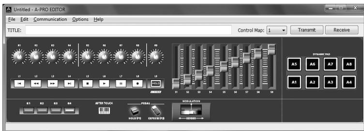
The A-PRO has a total of 44 controllers: [B1]–[B4], [R1]–[R9], [L1]–[L9], [S1]–[S9], [A1]–[A8], HOLD (P1), EXPRESSION (P2), BENDER, MODULATION, and AFTERTOUCH. You can freely assign any MIDI message to be controlled by each controller.
