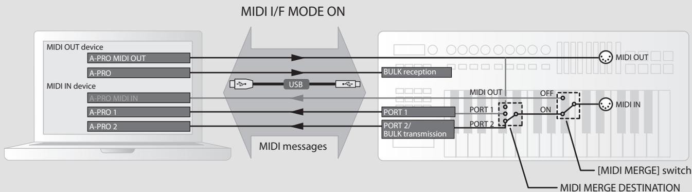
In this illustration, the [MIDI MERGE] switch is On and the MIDI MERGE DESTINATION is set to Port 2, so that messages received at MIDI IN are merged with the messages of Port 2 and sent to the computer.
