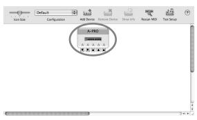
If the A-PRO is not shown or is grayed-out, the A-PRO has not been recognized correctly. Try clicking [Rescan MIDI]. You can also try disconnecting the USB cable connected to the A-PRO, then re-connecting it.
