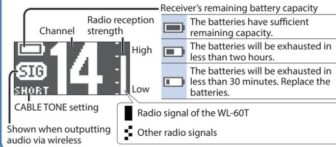
**Selecting the Receiver's Channel Automatically (Scan Mode)**
