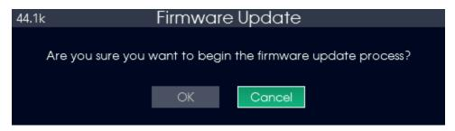
Select the "OK"indicator and press <u>Select</u>. The firmware update will progress through four stages: Erasing, Programing, Verifying, Complete
