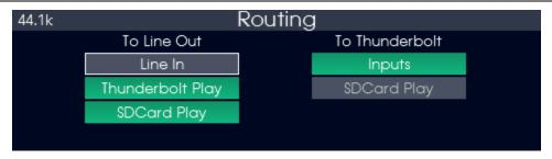
The "Routing" page is where you control what sources you are able to monitor and record. This page involves "global" routing. You can get more sophisticated, with per-channel routing, using the Lynx Mixer software when using the Thunderbolt connection method. This page, however, is ideal for setting source to destination for all channels quickly, or for setting up the Aurora<sup>(n)</sup>routing independently of the computer.
