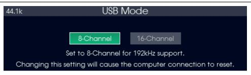
The Aurora<sup>(n)</sup>-16 USB has a unique page to itself. The LT-USB can operate in two different modes, 8-Channel and 16-Channel. In 8-Channel mode, 192kHz operation is possible, however in 16-Channel mode 96kHz is the maximum sample rate. This page allows switching between the two modes. Please note that changing the setting will reset the computer connection.
