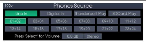
The Phones Source page can be brought up from any other page on the Aurora<sup>(n)</sup> display by simply pressing the <u>Phones Source</u> button. This is where the source can be selected for the two headphone outputs. Please note: The PHONES have independent level controls, but the source selected will apply to both jacks.
