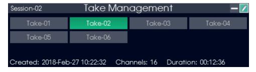
The <u>TakeManagement</u> page is where individual recordings can be managed. Each time the <u>Record</u> button is pressed, a new take is created in the current session using the settings from the <u>SD Record Setup</u> page. Each take is date and time stamped, and date and time is shown when the take is highlighted along with the number of channels and the duration of the take in HH:MM:SS format.
