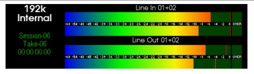
The horizontal meters show greater detail for two pairs of channels on the Aurora<sup>(n)</sup>. Level markers and clip indicators make this a useful tool for calibration and troubleshooting.
