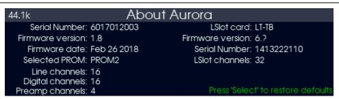
The "About" page is a convenient way to determine system specifics, such as firmware versions and dates, serial numbers and installed expansion cards. Pressing the <u>Select</u> button will restore the Aurora<sup>(n)</sup> to factory default settings.
