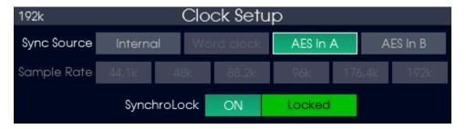
AES In A and AES In B will only be displayed when the LM-DIG board is installed in the Module 4 position. When clocked via AES Input, the Aurora<sup>(n)</sup> will follow whatever sample rate is being generated by the AES device feeding the selected input. It is critical that the clock master is generating the sample rate that matches the rate of your audio project, to prevent recording audio at the wrong pitch and speed.
