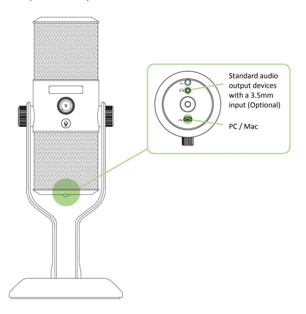
Note: By connecting an analog audio output device (such as a headphone) via the 3.5mm connector, you can listen to the audio being recorded by your Razer Seirēn as it happens. Note that this does not play any audio from the PC directly.
