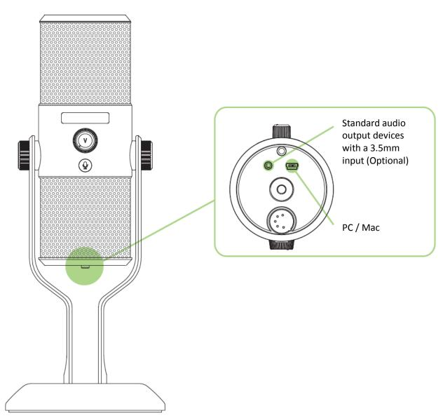
Note: By connecting an analog audio output device (such as a headphone) via the 3.5mm connector, you can listen to the audio being recorded by your Razer Seiren Pro as it happens. Note that this does not play any audio from the PC directly.
