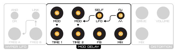
**(5) The TIME 1 and TIME 2** knobs set the delay time for each line.
