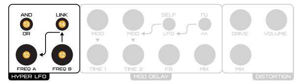
FREQ B. In upward position, FREQ A is multiplied by FREQ B, which is the logical operation AND. Both operations are conducted on a square waveform. The addition is analogue, and the LFO output signal has a gradient.
