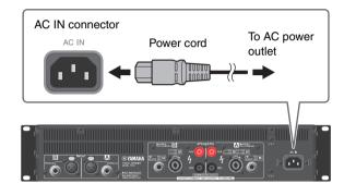
Secure the AC power cord with the AC plug clamp to prevent accidental disconnection from the connector.
