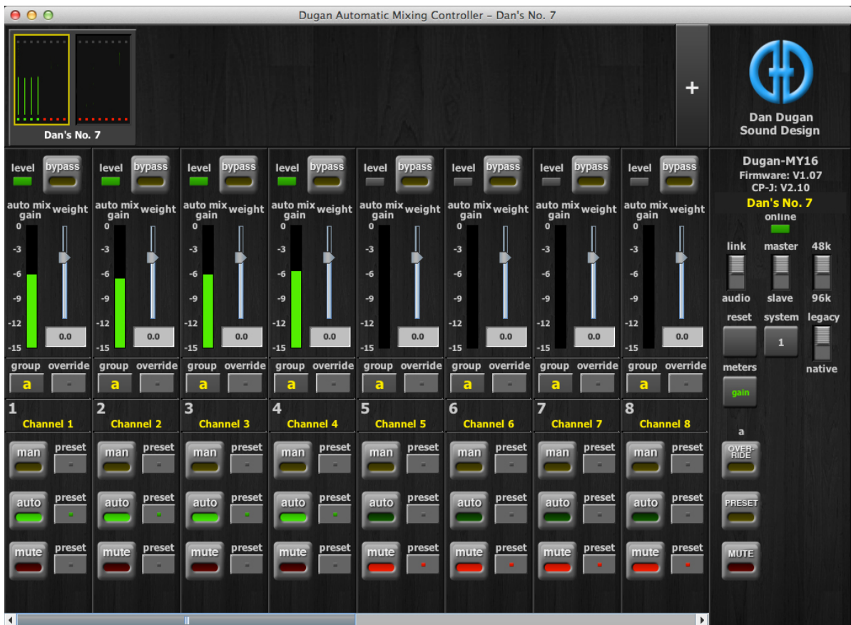
Figure 3-1 Dugan Control Panel
