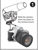
Before sliding the camera shoe into place, loosen the fastening ring by turning anti-clockwise until it is loose enough to fit easily into your camera's shoe mount. Once the shoe is in place, gently tighten by turning the fastening ring clockwise until the VM-6 is seated firmly in place.
