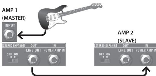
1. From the LINE OUT jack of the amp to which your guitar is connected (MASTER), connect to the POWER AMP IN jack of the other amp (SLAVE).
