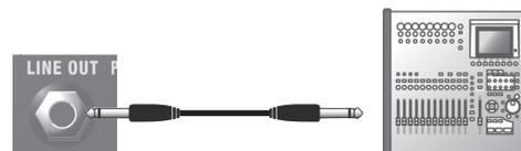
You can use this in conjunction with an external PA system, or to record your performance via direct line while monitoring the sound from the KATANA Mk II's speaker.
