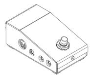
There's only one switch on the controller surface, it's here to put the Perc into a learning mode. Press the button for two seconds, the LED on the back panel will start flashing. Now the controller is in its learn mode and is waiting for a signal from your controlling device. This way Perc controller will learn the MIDI note and channel for its corresponding beater.
