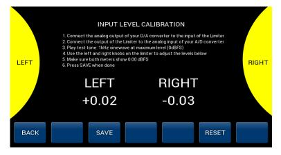
The mastering limiter is prepared to work straight form the box. In most cases the metering will be accurate and the limiter will behave perfectly. However if you would like to calibrate the 0dBFS reference with your D/A converter super precisely, we have added an option to do so.
