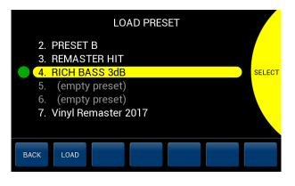
Loading presets is very simple too. Just Press **LOAD** in the Main Menu, choose the preset and hit LOAD in the LOAD PRESET window. The Mastering Limiter will recall all the settings and activate the ENGAGE. Press BACK or scroll thru other presets to find the one that suits your needs.
