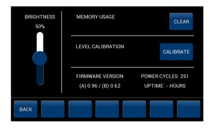
This screen allows you to adjust the BRIGHTNESS of the screen (touch and drag the virtual slider the screen), check on the firmware version of your unit, see the number of power cycles (how many times the unit was turned off and on), but also to **CLEAR** presets memory and the CALIBRATION perform procedure (it has to be done only once when you connect the
