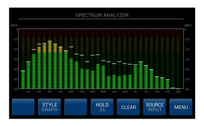
The spectrum analyzer window gives you a great, real-time insight into the current content of frequency the processed signal. By pressing **STYLE** button you the can choose two types of graphical to fulfill your representation needs. BARS style with 30 animated meters and peak hold functionality (you can personalize this feature by
