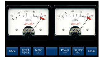
VU – Volume Unit Meter, calibrated to show 0dB when 0dBFS 1kHz sine signal is present. The fall time is the same as the integration time - 300 ms.
