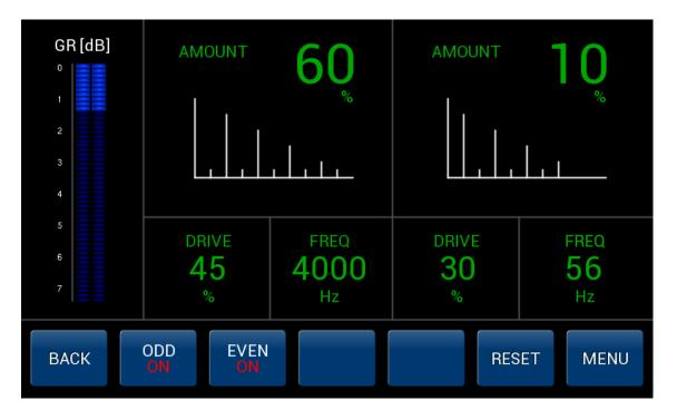
Use the ON/OFF buttons on the bottom of the screen to enable or disable one or both of the harmonic generators (colors). Press **RESET** to set the generators settings to their default values.
