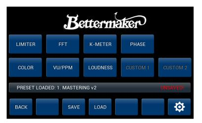
Here, you can either go back to the Limiter Window or go to the COLOR screen and adjust the settings of odd/even harmonics generator. You can also choose one of the measurement tools like FFT analysis, K-metering and other that will be explained in following chapters of this manual.
