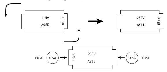
5. Place the cartidge back in the holder it so that the 230V value is displayed through the slot in the fastening. Re-seal the fastening, reconnect the IEC power cable, and switch the unit on.
