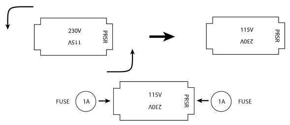
5. Place the cartidge back in the holder it so that the 115V value is displayed through the slot in the fastening. Re-seal the fastening, reconnect the IEC power cable, and switch the unit on.
