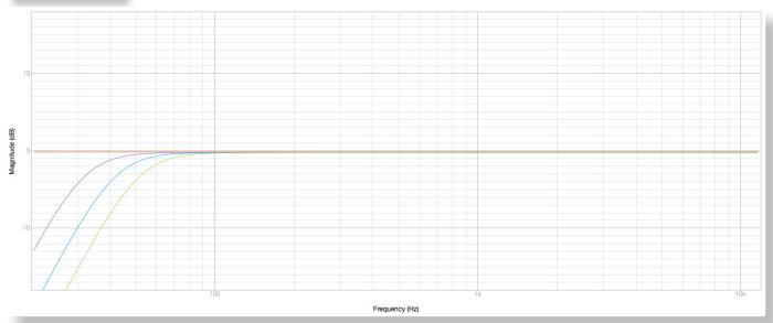
HPF Plots - OFF, 30Hz, 40Hz, 50Hz.
