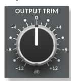
The **OUTPUT TRIM** provides ±12dB gain at the output stage of Fusion. This pot is indented at the 12 o'clock position. This control is important in order to compensate for any level increases caused by the preceding sections.
