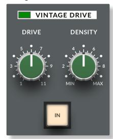
**VINTAGE DRIVE** is a unique, non-linear saturation circuit that gives your mix added strength and cohesion. This circuit has been designed to bring the kind of cherished 'gradual analogue overload' sound that the best kind of vintage analogue outboard and consoles offer when you drive level into the sweet spot.
