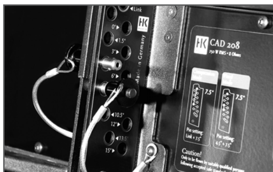
Fig. 20: Example of a fixed mode application with a 4.5° angle
