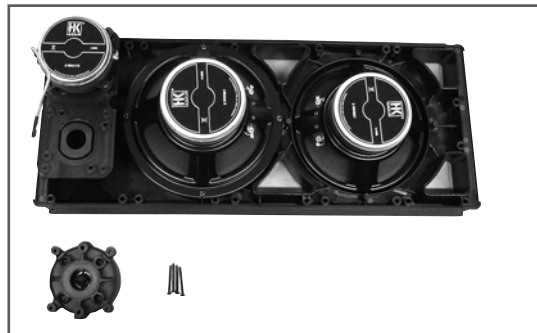
Fig. 37: Dismantled CAD 208 baffle board with the woofer
