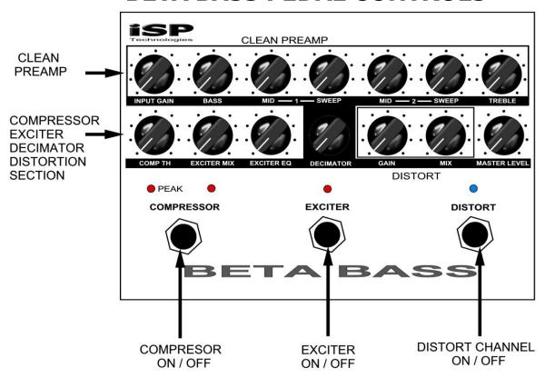
The upper row of controls are for the clean preamplifier. The lower row of controls are for the Compressor, Exciter, Decimator Noise Reduction and Distortion Circuit. Three footswitches are provided with the first footswitch allows the player to select Compressor ON / OFF. The second footswitch switches ON and OFF the Bass Exciter. The third footswitch switches ON and OFF the Distortion circuit.
