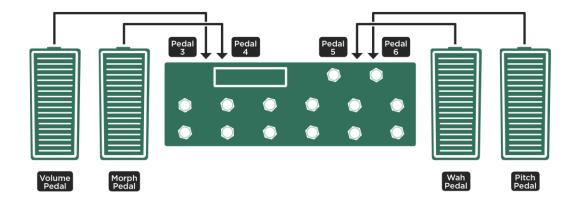
Four dedicated pedals connected to PROFILER Remote; for PROFILER Stage use PEDAL 1-4 plugs
