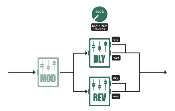
As you turn "DLY+REV Routing" more to the right, the opposite happens: the delay reflections keep their reverb tail, but the dry signal loses its reverberation and becomes completely dry. This will emphasize your instrument, as the reverb will not appear until after the first delay reflection.
