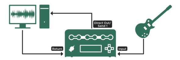
Reamping with analog connections
