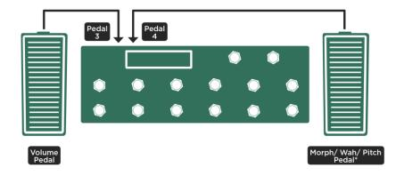
\*Morph Pedal also controlling Wah and Pitch ("MorphPedal to Wah" and "MorphPedal to Pitch"); Morphing triggered via buttons
