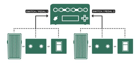
Connecting pedals and switches to PROFILER directly
