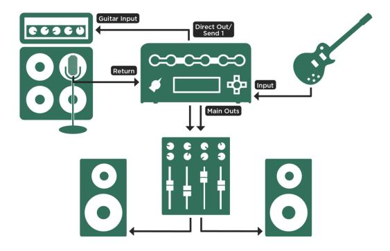
Normal connections; on PROFILER Stage connect to SEND 1 and RETURN 1
