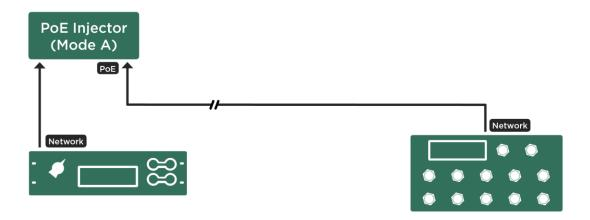
Cabling with PoE injector close to PROFILER
