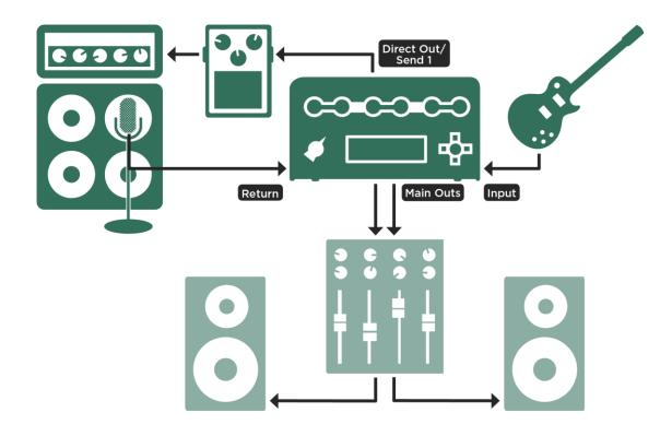
Connections including a stomp box; on PROFILER Stage connect to SEND 1 and RETURN 1
