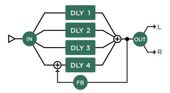
When you set Feedback to above zero, the whole delay pattern is repeated. The repetition time (and thus pattern length) is defined by the time of the fourth delay tap (Delay 4). For that reason, the fourth delay tap is always the first tap of the next repetition.
