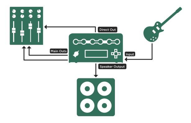
Wet-dry-wet connections with PowerHead or PowerRack
