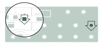
It also works the other way around: press and hold the module button on the PROFILER first, then step on the desired Effect Button afterwards. The upper left LED of the Effect Button should now reflect the <u>category color of the effect</u> you assigned e. g. orange for a wah effect. Now, you can activate or bypass the selected effect module by stepping on the button on your PROFILER Remote. The lower left white LED indicates the on/off status of this effect module.
