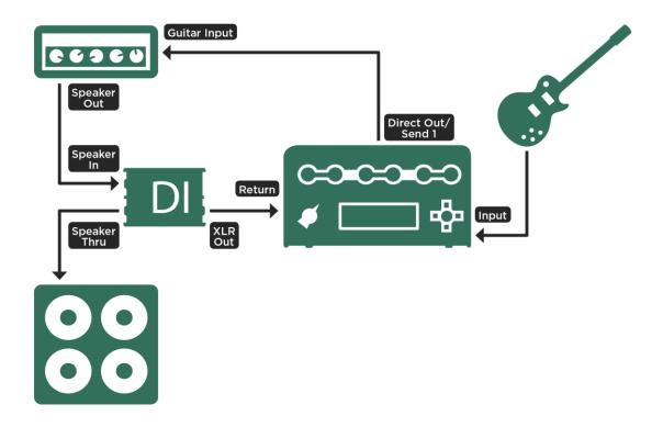
Capturing a Direct Amplifier PROFILE; on PROFILER Stage connect to SEND 1 and RETURN 1
