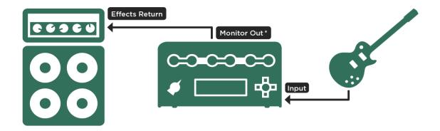
\* Cabinet simulation deactivated for Monitor Out
