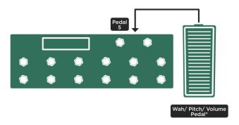
\* Wah Pedal also controlling Pitch and Volume ("WahPedal to Pitch" and "WahPedal to Volume"); Morphing triggered via buttons
