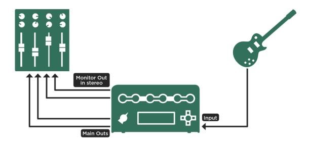
Wet-dry-dry-wet connections with Monitor Stereo
