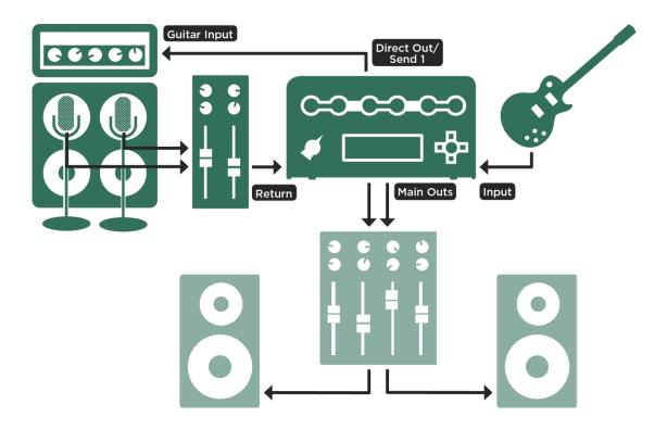
Connections with multiple microphones; on PROFILER Stage connect to SEND 1 and RETURN 1
