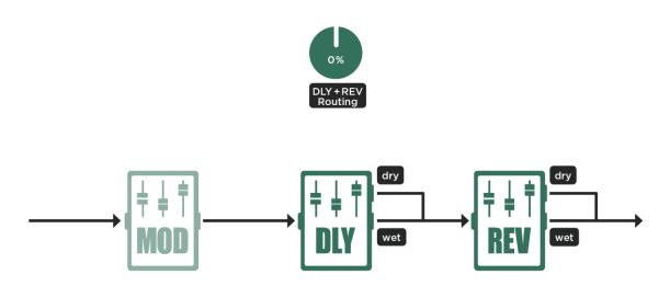
When you turn "DLY+REV Routing" more to the left, you will notice that the delay reflections will vanish from the reverb - at fully left position, only the dry portion of the delay gets reverberated. Now, the delay and reverb are working in a parallel configuration. You will hear delay reflections and a reverb tail, but the delay signal doesn't feed the reverb.
