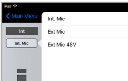
Select the Analog Level setting that corresponds to the input source you'd like to record. For example, if you have a microphone connected to the XLR connection on the breakout cable, select **Ext Mic** from the Analog Level menu on channel 1. If you would like to utilize ONE's built-in microphone, select **Int Mic**. By default, the 1/4" instrument input is the selected source for Channel 2.
