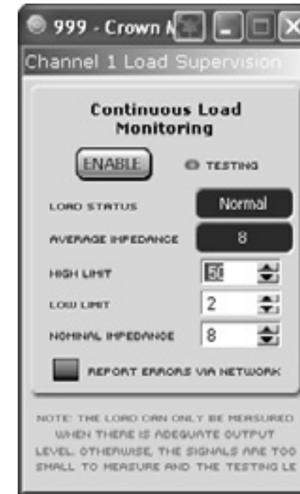
Figure 4.6 MA-i Load Monitoring Panel
