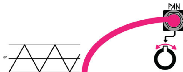
Bipolar control voltage is added to and subtracted from the position of the panel control. Panel control is set to 12:00 for modulation around the center.
