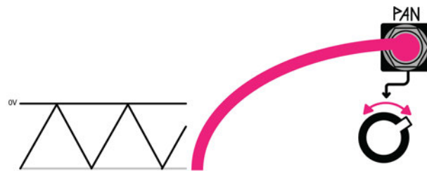
Negative control voltage is subtracted from the position of the panel control. Panel control is set clockwise for modulation around the center.
