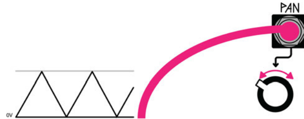
Positive control voltage is added to the position of the panel control. Panel control is set counterclockwise for modulation around the center.
