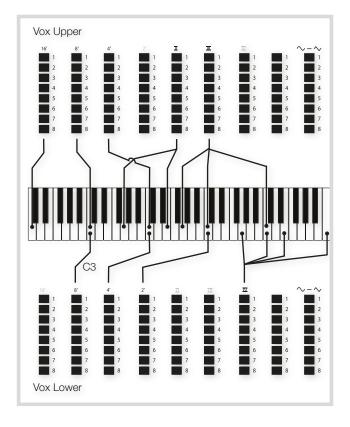
The rightmost drawbar controls the mix between a filtered signal sounding soft and dark, and an unfiltered signal sounding bright and intense.
