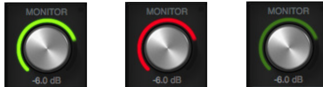
Monitor level indications (from left to right): Normal, Mute, and DIM/MONO
