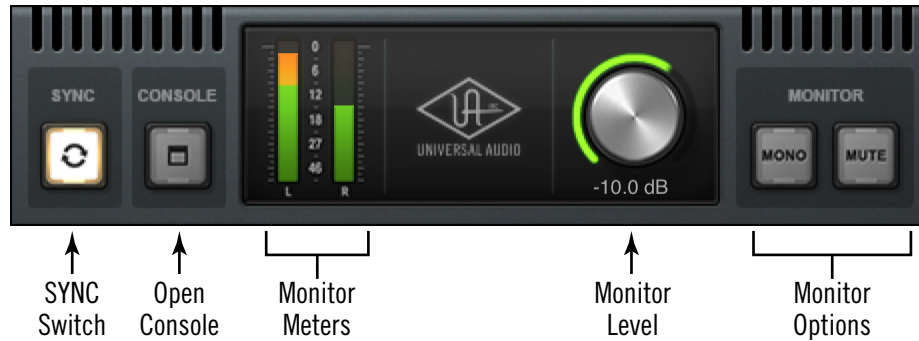
Console Recall plug-in controls
