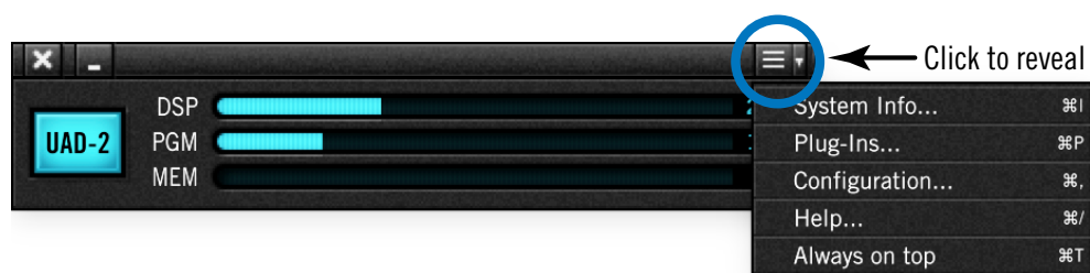
Control Panels drop menu
