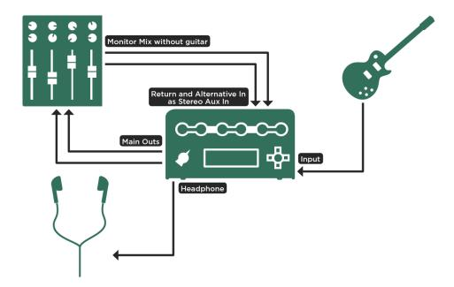
Mixing guitar signal with monitor mix locally; PROFILER Stage: use RETURN 1 and 2 jacks for Aux In
