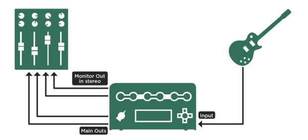
Wet-dry-dry-wet connections with Monitor Stereo
