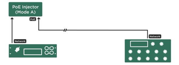
Cabling with PoE injector close to PROFILER
