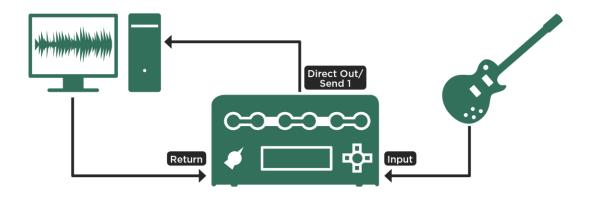
Reamping with analog connections
