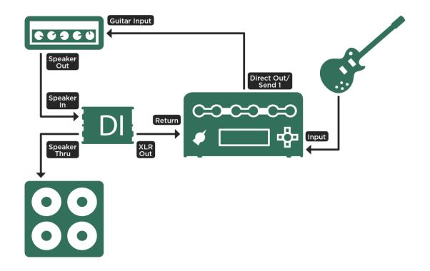
Connections PROFILING with DI; on PROFILER Stage connect to SEND 1 and RETURN 1
