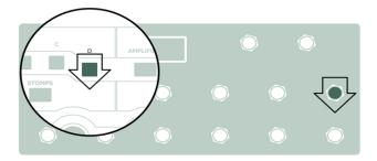
It also works the other way around: press and hold the module button on the PROFILER first, then step on the desired Effect Button afterwards. The upper left LED of the Effect Button should now reflect the <u>category color of the</u> <u>effect</u> you assigned e.g. orange for a wah effect. Now, you can activate or bypass the selected effect module by stepping on the button on your PROFILER Remote. The lower left white LED indicates the on/off status of this effect module.
