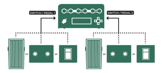
Connecting pedals and switches to PROFILER directly
