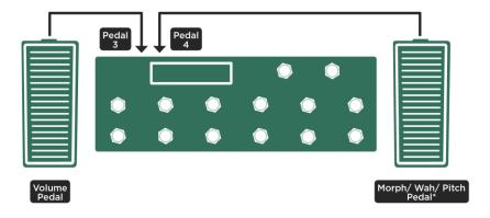
One dedicated pedal for volume and the Morph Pedal to be shared for wah and pedal pitch effects; for PROFILER Stage use PEDAL 1+2 jacks
