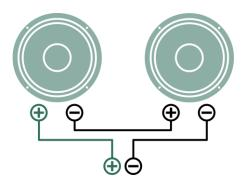
Running two KEMPER Kones in series, resulting in 8 ohms
