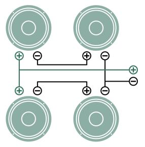
Running four KEMPER Kones in parallel/serial configuration, resulting in 4 Ohm
