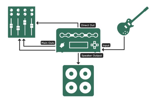
Wet-dry-wet connections with PowerHead or PowerRack
