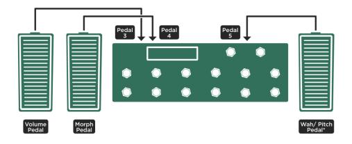
Two dedicated pedals for volume and Morphing plus one shared pedal for wah and pedal pitch effects; for PROFILER Stage us PEDAL 1-3 jacks
