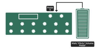
One wah pedal to be shared for volume and pedal pitch effects; for PROFILER Stage use PEDAL 3
