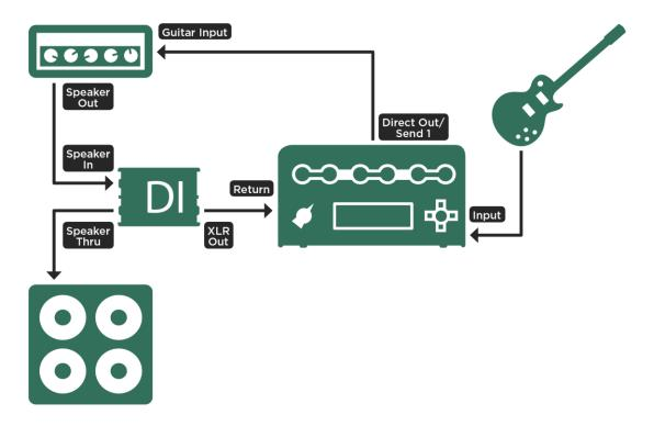
Capturing a Direct Amplifier PROFILE; on PROFILER Stage connect to SEND 1 and RETURN 1
