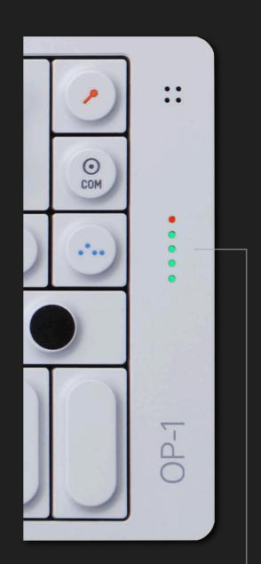
The Battery level is indicated by the LED array on the right side of your OP-1. All LEDs lit (including the red) indicates a fully charged battery good for around 16 hours of heavy use. The stand-by time is approximately 2 years.
