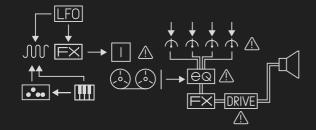
NOTE: A warning symbol will light up when any critical level is set to zero.
