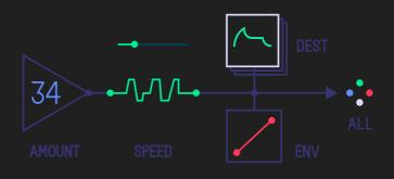
Blue encoder sets Amount. Green encoder sets speed. White sets Destination and Orange encoder sets the envelope Attack/Decay.
