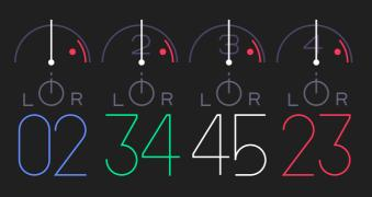
In the Mixer main screen, you adjust the individual level and Pan Left/Right of Tape tracks 1-4
