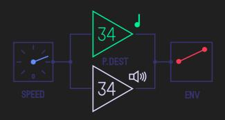
Blue encoder sets Speed. Green encoder sets Pitch. White encoder sets Volume and Orange encoder sets the envelope Attack/Decay.
