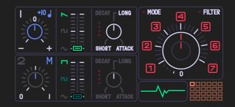
DBOX, short for DRUMBOX, is a dual oscillator synthesizer, convenient for producing drum sounds. Blue encoder adjusts pitch, Green encoder adjusts waveform, White encoder adjusts envelope. Hold SHIFT to access secondary oscillator. Orange encoder is used for Cross Modulation and, when SHIFT is pressed, Filter cutoff frequency.
