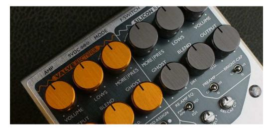
Remember that, regardless of which rectifier you use or where you set the GHOST control, the amount of sag you experience will always depend on how hard you are working the power stage. Sag occurs when the power amp is asking for more current than the power supply can, at that moment, deliver. The amount of sag, and its onset and recovery characteristics, will therefore depend on the level of your input signal, how hard you play and how high the VOLUME knob is set.
