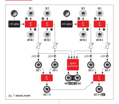
The motivation of this setup is that besides typical processing of external signals, it allows sampling of manually controlled voltages when offsets (either positive or negative) in channel **1** and **3** are engaged.
