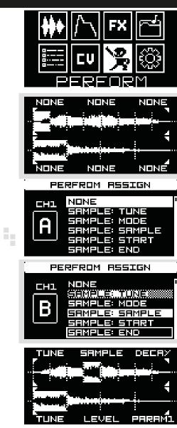
The PERFORMANCE mode is dedicated interface to use the Sample Drum in live performances. Once you have completed sample management (adjusting start/loop/end points or slicing), CV assign and applied FXes on both channels, in the Performance screen you will see both samples associated with the project with slices applied and also CV mappings for both channels are active.
