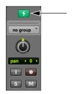
Track DSP Mode button enabled: in the Edit window (left) and in the Mix window (right)
