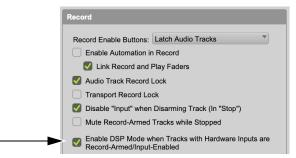
Enable DSP Mode when Tracks with Hardware Inputs are Record-Armed/ Input-Enabled option selected
