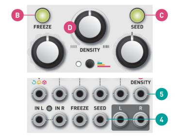
In this mode, the grains are generated continuously, at a rate set by the **DENSITY** knob [D] and modulated by the **DENSITY** CV input (5).
