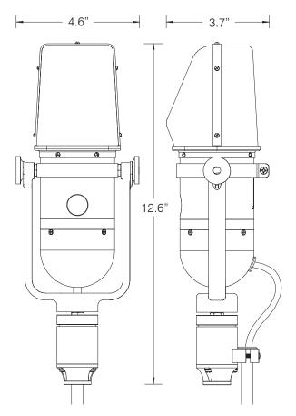
KU4 weight with cable: 4.7 pounds (2.15 kg) KU4 weight with case: 7 pounds (3.2 kg) Length: 12.65 in (32.4 cm) Width: 4.62 in (11.7 cm) Depth: 3.75 in (9.5 cm)
