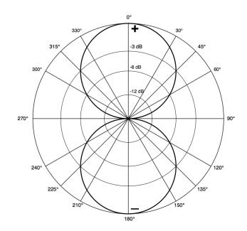
The AEA KU4 is unlike any other ribbon microphone, because its polar response has been tailored to provide a supercardioid pickup pattern.
