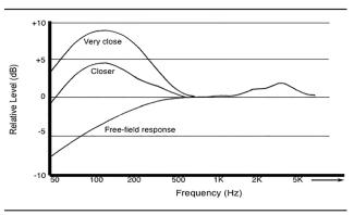
Proximity effect, a characteristic of all directional microphones, is a rise in low-frequency response at closer working distances. This can be used to superb effect, particularly with deeper vocals to enhance richness and depth. A potential trade-off is reduced articulation resultant of the masking effect on the treble due to "excessive" bass boost.
