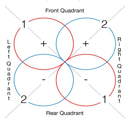
The front quadrant (pictured above) is the positive polarity stereo image, and the rear quadrant is the negative polarity stereo image. This is the stereo equivalent of the difference in sound between speaking into the front and rear of a bidirectional; the recording sounds as if it is coming from behind you. What is physically happening in a negative polarity recording is that the impulse that would usually push air towards your ears is now pulling air away from your ears.
