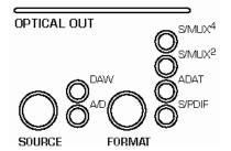
The optical output can provide either AES/EBU or ADAT format. The AES/EBU mode works with most S/PDIF optical inputs.
