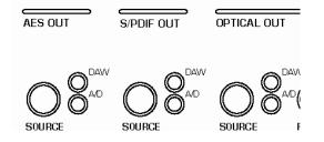
The digital outputs can stream digital audio data from either the ADC16's internal A/D converters or from the source connected to the optional 'DAW' interface card.
