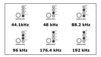
The 'SAMPLE RATE' LED display always indicates the sample rate at which the ADC16 is operating.
