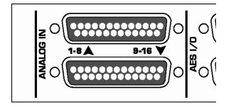
The balanced "ANALOG IN" line-level inputs follow the Tascam Analog DB-25 standard. Cables are available from many sources.
