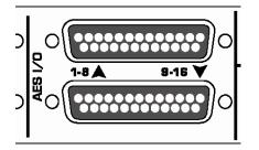
The balanced 'AES I/O' digital I/O connectors follow the Tascam AES/EBU DB-25 standard. Cables are available from many sources.
