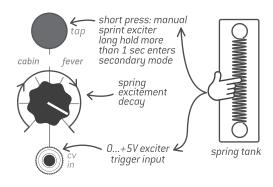
the spring sounds long (up to infinite) with a small self-oscillation. Keep that in mind when you select this effect.
