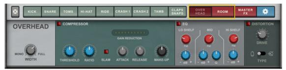
The Overhead and Room mics sections feature identical modules, that can be used for shaping the sound from the overhead and room microphones respectively.
