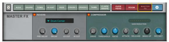
The Master FX section features a convolution Reverb, which is routed as a send effect for the channels in the Mic Mixer, as well as for the Tambourine and Claps & Snaps instruments. It also features a Compressor routed as a master insert effect, to affect the entire output mix.
