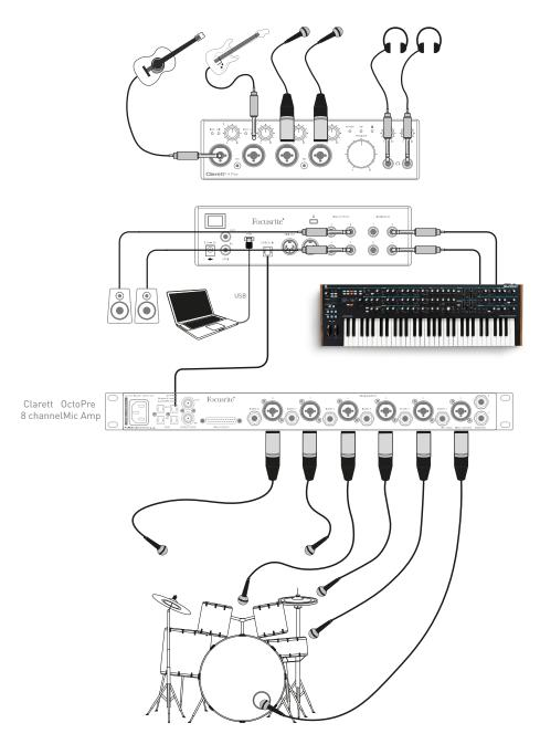
The Clarett OctoPre's **OPTICAL OUT** port is connected to the Clarett+ 4Pre's **OPTICAL IN** port with a single TOSLINK optical cable. The two devices must be synchronised to ensure audio passes cleanly, without clicks and pops. To do this in **Focusrite Control** go to **Device Settings** and set the **Clock Source** to **ADAT**. Both devices must be set to the same sample rate.
