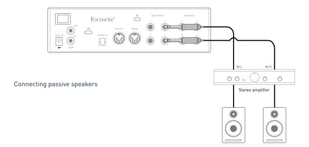
Professional power amplifiers will generally have balanced inputs. If your amplifier or powered speakers have balanced inputs, use 3-pole (TRS) 1/4" jacks to connect them to the Clarett+ 4Pre.
