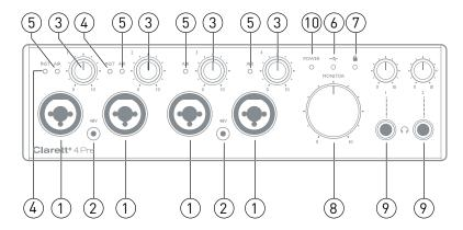
The front panel includes input gain controls and input connectors for Mic, Line and Instrument signals for both channels, and also monitoring controls.
