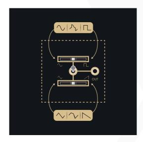
Oscillator 1: If the Waveform Selection Toggle is in the up position, the signal present at the Waveform Output will smoothly morph between a sine waveform and a triangle waveform as the Waveform Crossfader moves from left to right. If the Waveform Selection Toggle is in the down position, the signal present at the Waveform Output will smoothly morph between a ramp waveform and a square waveform as the Waveform Crossfader moves from Crossfader moves from left to right.
