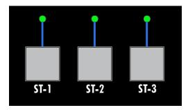
To select an analog input source, press the desired **ST-1**, **ST-2**, or **ST-3** source selector button:
