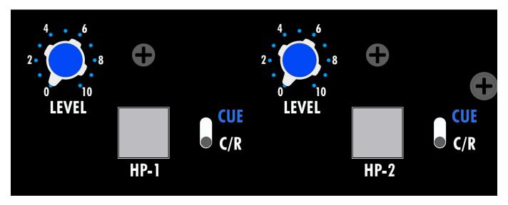
The MC531 is equipped with two independent stereo headphone amplifiers, HP-1 and HP-2. The amplifier circuit is the same as found in API consoles such as THE BOX, 1608, 1608-II, and 2448.
