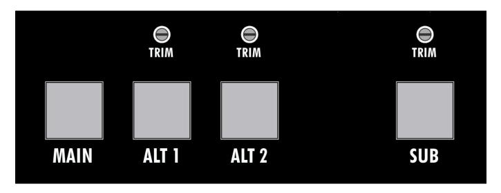
The MC531 supports three (3) sets of stereo audio monitors, plus a subwoofer with a programmable link to each stereo pair. Only one set of monitors can be selected at a time.
