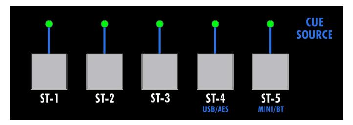
Five (5) input source selectors provide a choice of seven (7) different audio sources to feed the selected set of monitors. Each input source is buffered with an API 2510 op-amp. Only one source can be selected at a time.
