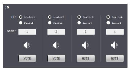
Signal source input: analog input signal or Dante input signal
