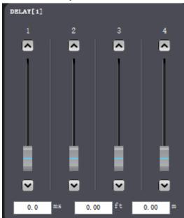
Delayer: adjust the signal delay of the corresponding channel through the fader (0~60ms)
