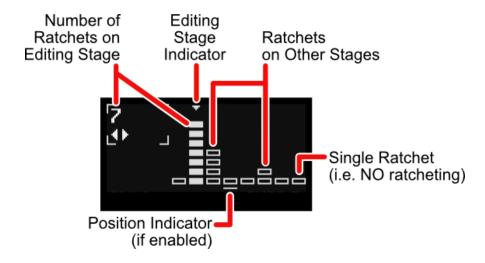
Each stage has a ratchet count from 1 to 8, and the interpretation of this count depends on whether or not **Gate Stretching** (as set in the <u>Track Menu</u>) is <u>ON</u> or <u>OFF</u>, as discussed later in this section.
