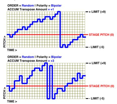
NOTE: Since the 'drunken walk' can extend both above and below the stage pitch, and accumulations wrap to the opposite limit (rather than back to the stage pitch), this can result in some wider pitch swings — particularly when the 'walk' occurs near a limit.
