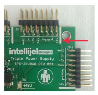
The other end of the cable, with a 16-pin connector, connects to the power bus board of your Eurorack case. Ensure the red stripe on the cable lines up with the -12V pins on the bus board. On Intellijel power supplies the pins are labelled with the label "-12V" and a thick white stripe. Sometimes the connectors are shrouded, ensuring the cable can only be oriented in one direction.
