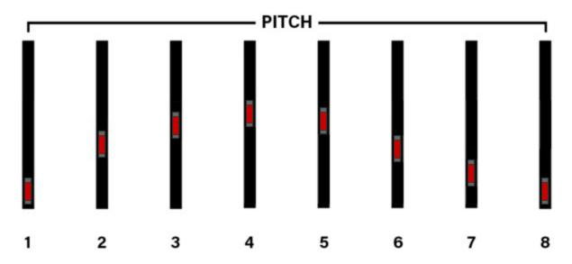
These sliders determine the default pitch value of each corresponding stage. Metropolix uses the position of these sliders as a starting point for determining the actual pitch output by each stage on each track.
