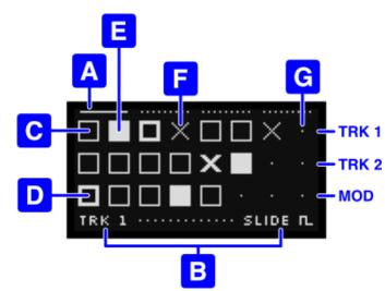
white block indicates the current stage **[E]**. An X indicates that a stage will be **skipped [F]**. A black stage block indicates the stage will play as expected. A black stage block with a thick outline **[D]** indicates the track's starting stage, as set with the **LEN** button's OFFSET parameter. If a track has a length shorter than 8 stages, a dot **[G]** is displayed for the unused stages.
