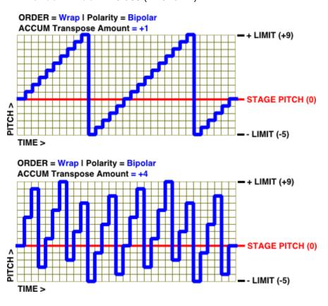
Pendulum Pitch accumulates in the direction set by the stage's TRANSPOSE AMOUNT. When the accumulated pitch reaches its Positive Limit (or Negative Limit), it reverses direction and continues accumulating in the opposite direction until it reaches either:
