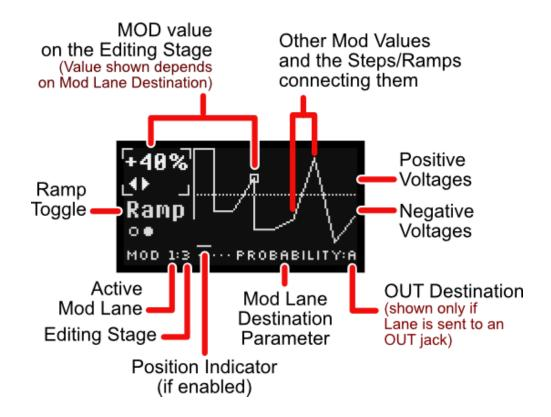
NOTE: If you have not yet assigned a MOD Lane Destination (discussed in <u>Assigning a MOD Lane to an Internal Parameter</u>), or if you assigned it to OUT A or B, the editable MOD Value range is +-5.00 V. If the MOD Lane destination controls a variable parameter (rather than a gated parameter), then the MOD Lane Edit Screen works as shown above. If you've assigned a MOD Lane to a gated destination, the MOD Lane Edit Screen works as described in <u>Editing</u> <u>Gates in a MOD Lane</u>.
