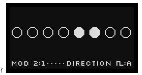
Each MOD lane can have its own playback ORDER, LENgth and clock DIVision, but the three track timing buttons (SWING, SLIDE and GATE) are not used.
