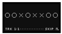
When SKIP is enabled for a stage, the sequencer treats the stage as if it did not exist — jumping past it to the next stage in the sequence (as defined by the <u>ORDER</u> screen). The stage's PULSE COUNT is also ignored completely, and does not count toward the total number of pulses in the sequence length.
